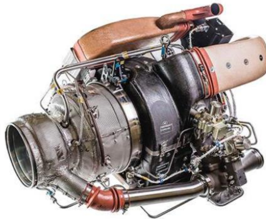
Gambar 1 Auxiliary Power Unit APS3200[7]
