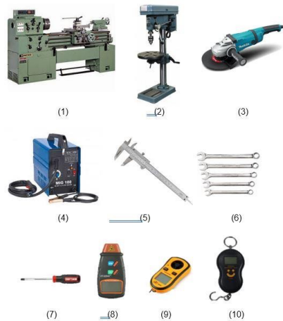
Gambar 2.1 Alat-alat Pendukung perancangan dan menghitung spesifikasi engine : (1) Lathe Machine , (2) Drill Machine , (3) Gerinder , (4) Welding Tools , (5) Vernier Caliper , (6) Wrench , (7) Srew Driver , (8) Thacometer , (9) Anemometer , (10) Digital Scale .
