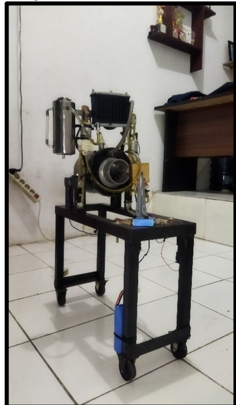
Gambar 2.10 Micro Turbojet Engine Aero-16
