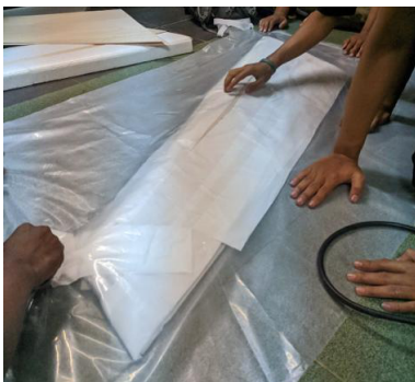
Gambar 4.23 Proses Vaccum Bagging
