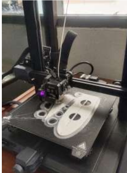
Gambar 4 Proses Pencetakan 3D Printing [6].
